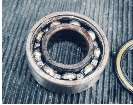
Figure 9: A degraded bearing (image courtesy of Aingura IIoT).
